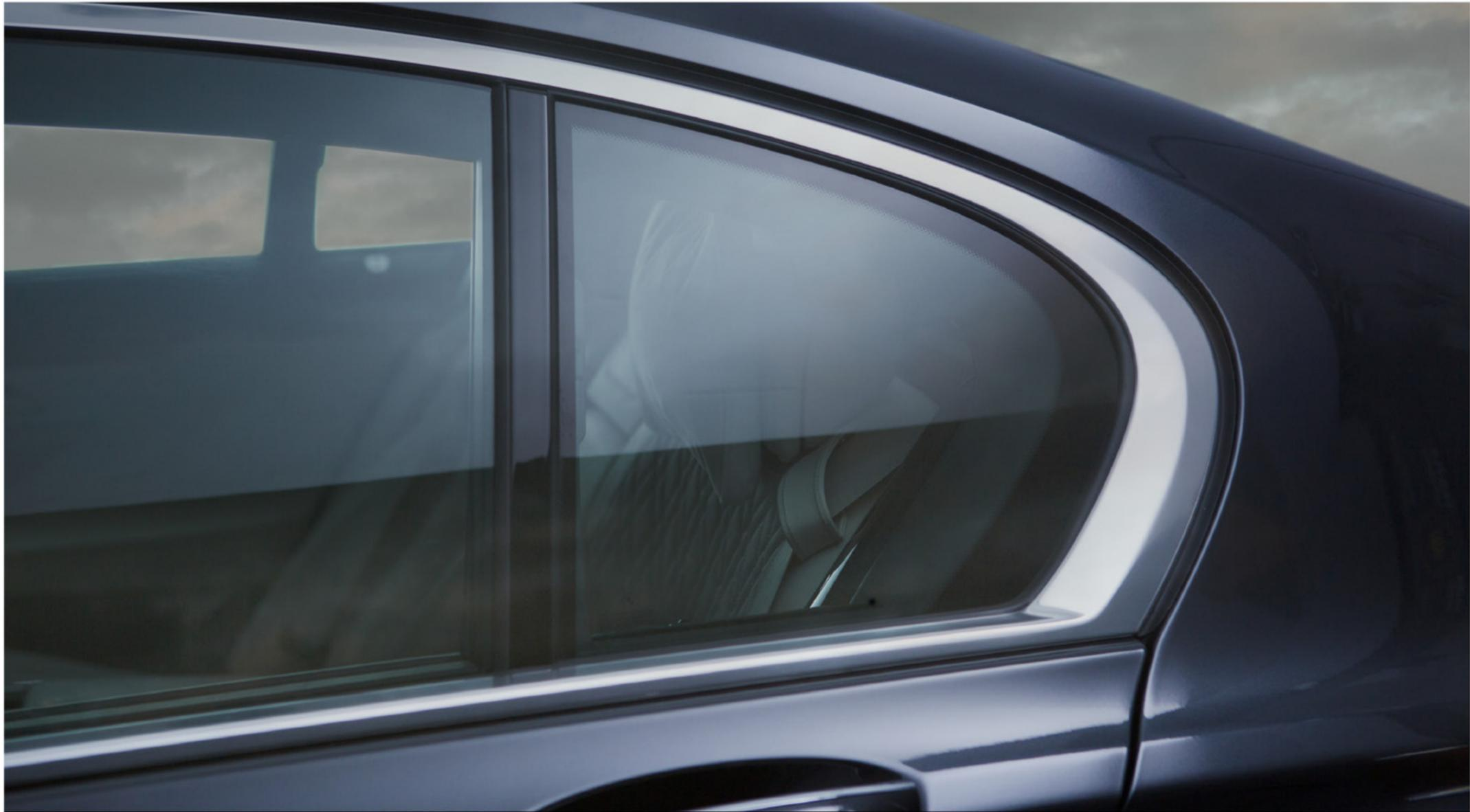
An iconic feature of BMW's design heritage, the Hofmeister kink in the new 7 Series is seamlessly incorporated into the window frame as a single-piece element.
